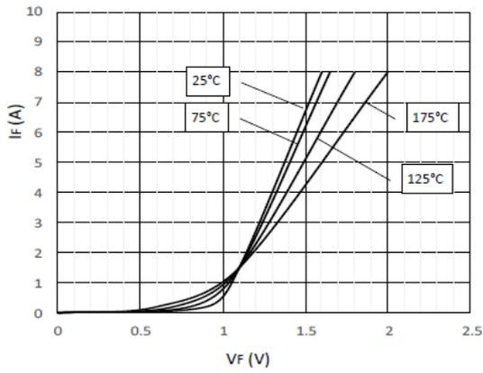
Fig 2. Diode forward current
